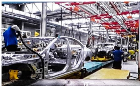
Process to join all the CKD components in the welding workshop
