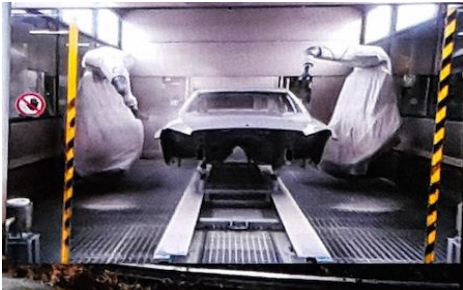
Painting the major body components in the paint workshop
